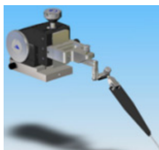
Picoprobe high impedance probe on DPP2xx-PTH positioner
